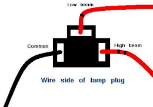
If you have a different type of Headlight connector, you may need an electrical manual, or you can use a voltage tester to confirm which wire is live when the High Beam is engaged. Also you can try Googling “headlight plug *then your model bike*” and often you will find the answer.
